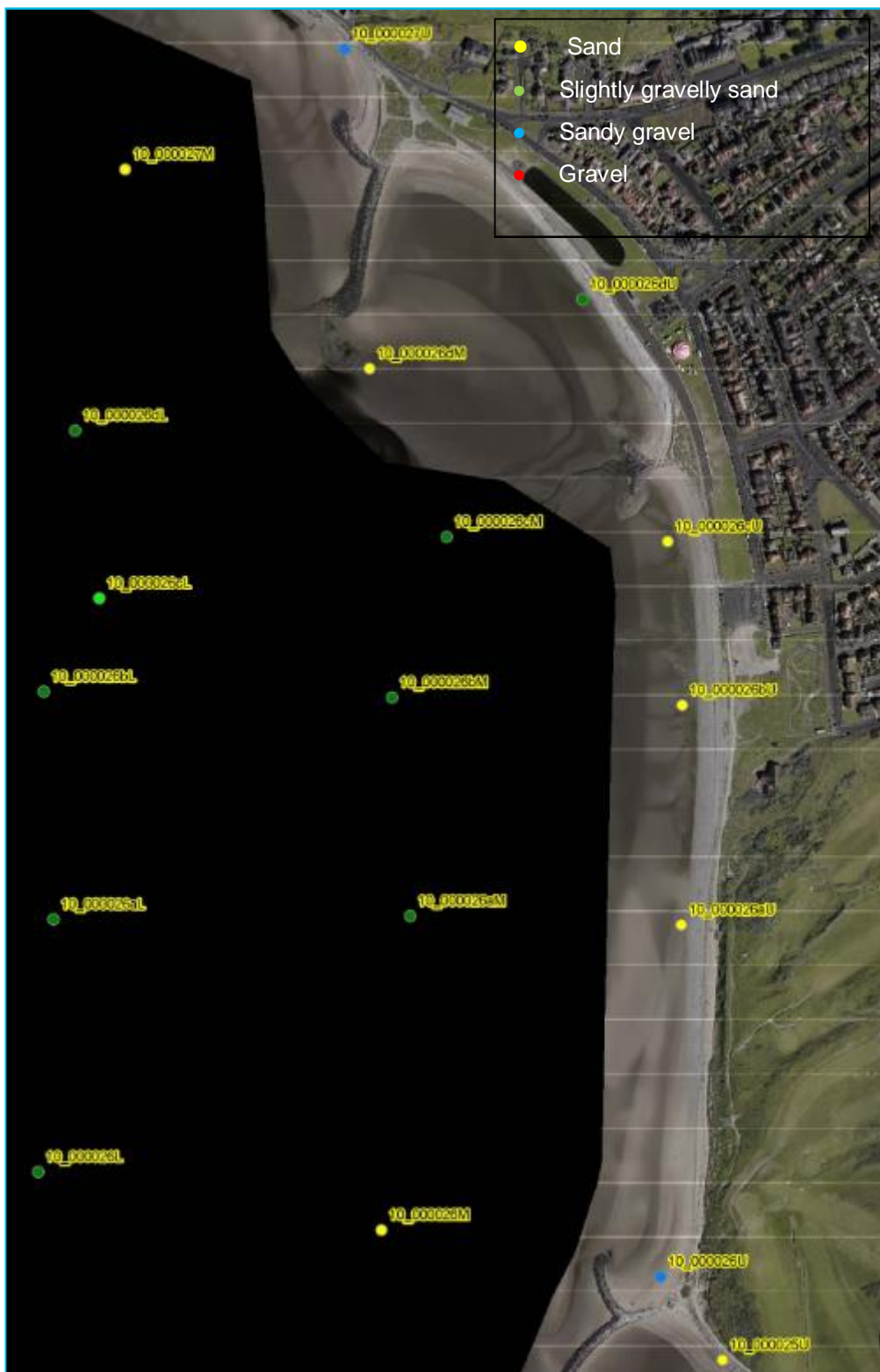
Figure 2.19 – Sediment sampling locations and sediment types recorded – West Shore
